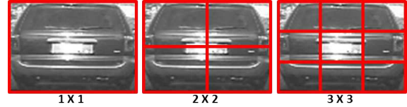
Figure 2. The spatial layout for local patches sampling. Note that, any other local patch sampling methods can also be adopted.
