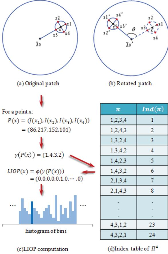
Figure 2. The construction of the proposed LIOP descriptor.
