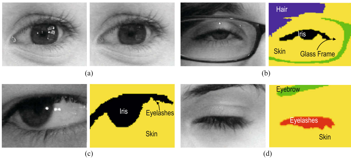
Fig. 6. Illustrations of (a) specular reflection removal and (b)–(d): clustering based coarse iris localization.
