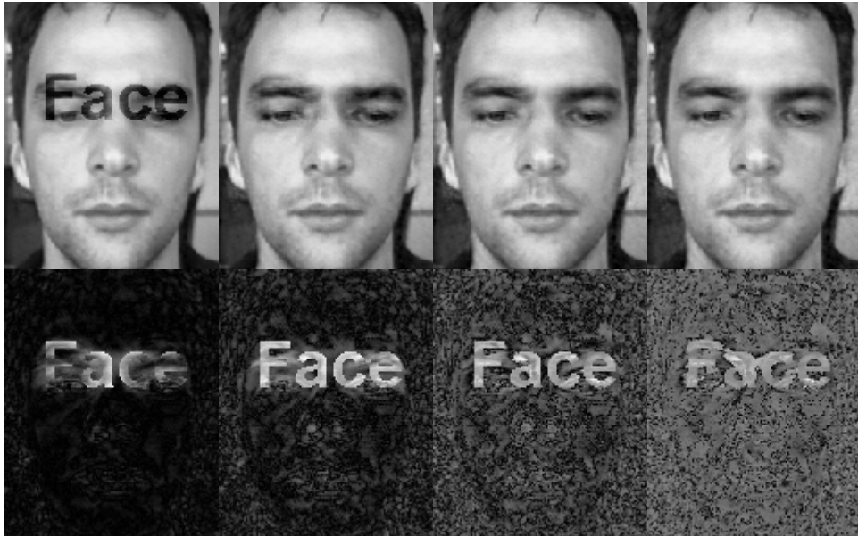
Figure 2: Reconstructed face and normalized successive error in step (1,3,5,7) with classical iterative PCA
