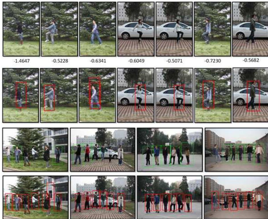
Fig. 11. (best view in color) 1st row: missed positive samples by HOG and their scores. These samples are with large pose variation. 2nd row: detection results by our method. 3rd row: detection results on multi pedestrians images by HOG. 4th row: detection results on multi pedestrians images by our method.
