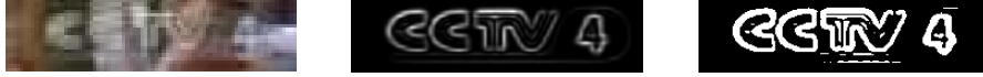
Fig. 2. TV logo mask extraction (Left to right: a frame from the original sequence, the generalized gradient image, and the logo's binary mask by OTSU algorithm)
