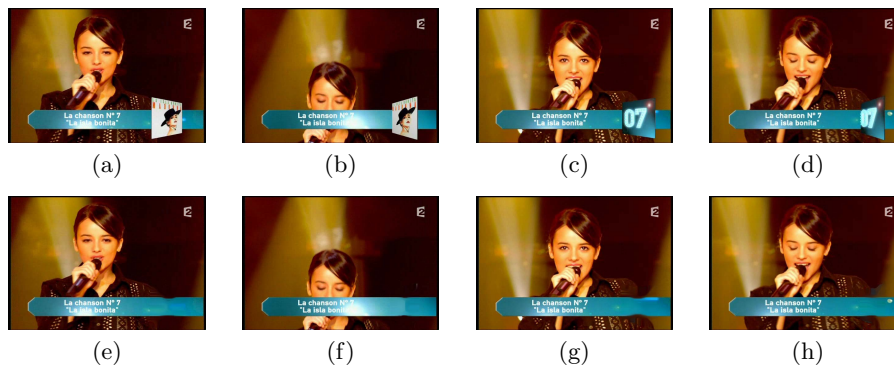
Fig. 6. Examples of TV logo removal for animated logos. Four logo templates that are obtained by difference of logo images are used to model the animated logo. (a), (b), (c) and (d) are frames with the animated logo. (e), (f), (g) and (h) are frames with removed logos with the regularization PDEs based approach.
