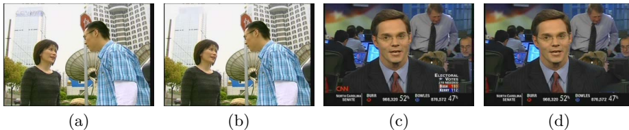
Fig. 3. Examples of TV logo removal based on the regularization PDE. (a) and (c) are original frames with TV logos. (b) and (d) are frames with removed TV logos.
